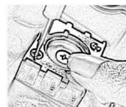
Tighten the lock screw in clockwise direction
