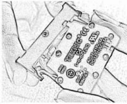
Snap fit the element by simple push action
