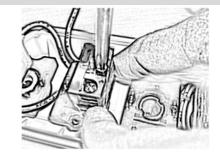
Tighten the Element screw with a screw driver with a torque of 0.5Nm in clockwise direction.
