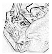
Tighten the Element screw with a screw driver with a torque of 0.5Nm in clockwise direction.
