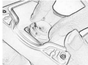
Tighten it with a torque of 2Nm
